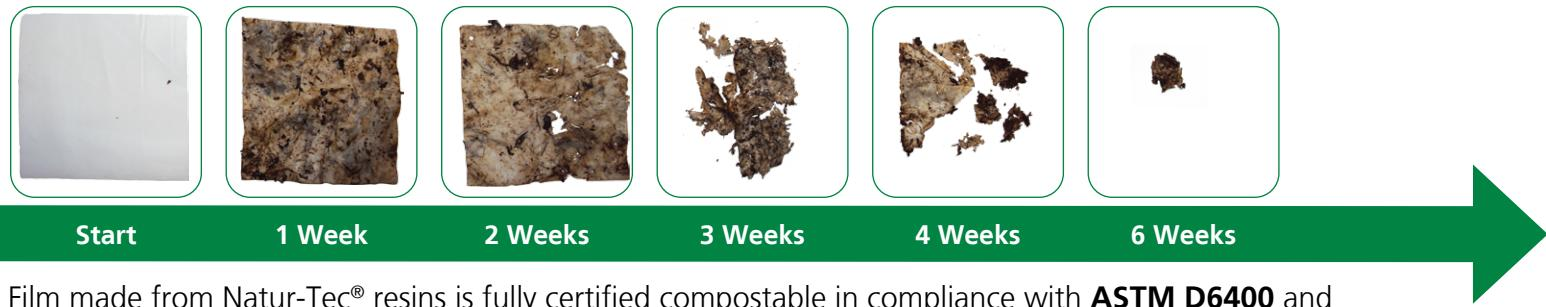
Film made from Natur-Tec® resins is fully certified compostable in compliance with **ASTM D6400** and **EN13432**. Composting is the biological process of breaking up organic matter such as food, food scraps, leaves, grass trimmings, paper, bioplastics, and more, resulting in biomass (nutrient-rich soil amendments).
